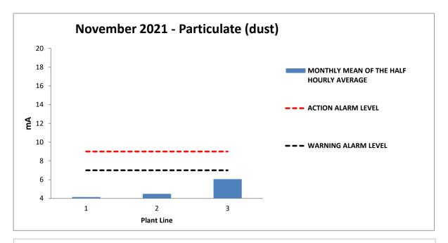
Following EA guidance and approval in July 2015, RRRL now monitor particulate emissions qualitatively as opposed to quantitatively. The particulate data is now reported in mA (milliamps) and the reporting range of the instrument is 4mA to 20mA where 4mA = 0 particles. The Half Hourly and Daily ELVs no longer apply, the ELVs have been replaced by two alarm levels that prompt the operator to start an investigation or take further action these are set at: 7mA – Warning Alarm and 9mA – Action Alarm.
