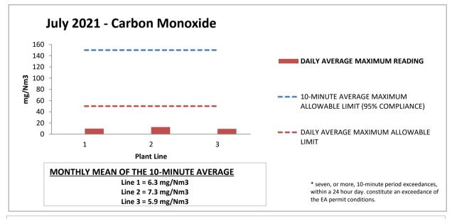
Following EA guidance and approval in May 2019, RRRL no longer report carbon monoxide against a half-hourly emissions limit value. Carbon monoxide is now monitored against the requirement to be 95% compliant against a 10-minute average value, of 150mg/Nm3, over a 24-hour period. Any 24-hour period where the 95% compliance level is breached will be highlighted in the chart above. The daily average emissions limit value of 50mg/Nm3 remains unchanged.
