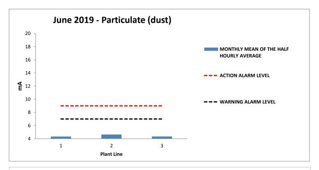
Following EA guidance and approval in July 2015, RRRL now monitor particulate emissions qualitatively as opposed to quantitatively. The particulate data is now reported in mA (milliamps) and the reporting range of the instrument is 4mA to 20mA where 4mA = 0 particles. The Half Hourly and Daily ELVs no longer apply, the ELVs have been replaced by two alarm levels that prompt the operator to start an investigation or take further action these are set at: 7mA – Warning Alarm and 9mA – Action Alarm.
