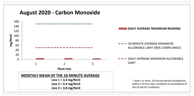
Following EA guidance and approval in May 2019, RRRL no longer report carbon monoxide against a half-hourly emissions limit value. Carbon monoxide is now monitored against the requirement to be 95% compliant against a 10-minute average value, of 150mg/Nm3, over a 24-hour period. Any 24-hour period where the 95% compliance level is breached will be highlighted in the chart above. The daily average emissions limit value of 50mg/Nm3 remains unchanged.
