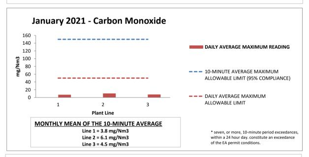
Following EA guidance and approval in May 2019, RRRL no longer report carbon monoxide against a half-hourly emissions limit value. Carbon monoxide is now monitored against the requirement to be 95% compliant against a 10-minute average value, of 150mg/Nm3, over a 24-hour period. Any 24-hour period where the 95% compliance level is breached will be highlighted in the chart above. The daily average emissions limit value of 50mg/Nm3 remains
