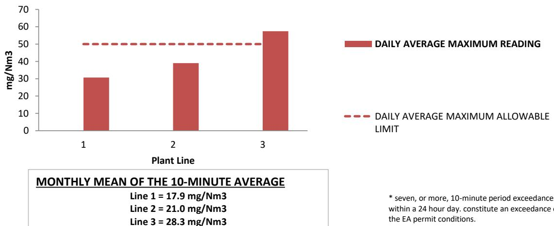
Following EA guidance and approval in May 2019, RRRR no longer report carbon monoxide against a half-hourly emissions limit value. Carbon monoxide is now monitored against the requirement to be 95% compliant against a 10-minute average value, of 150mg/Nm<sup>3</sup>, over a 24-hour period. Any 24-hour period where the 95% compliance level is breached will be highlighted in the chart above. The daily average emissions limit value of 50mg/Nm<sup>3</sup> remains unchanged.
