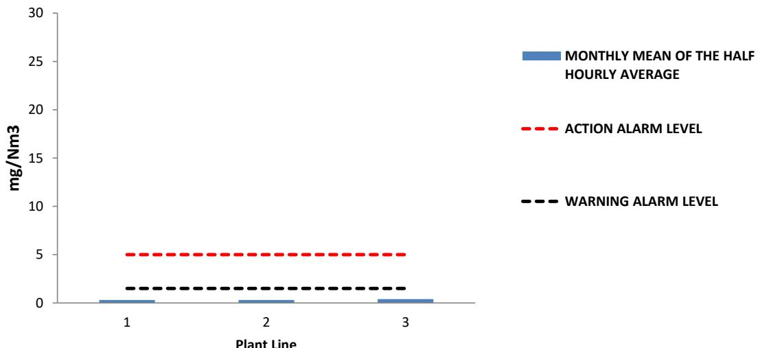
Following EA guidance and approval in July 2015, RRRRL now monitor particulate emissions qualitatively as opposed to quantitatively. The Half Hourly and Daily ELVs no longer apply, the ELVs have been replaced by two alarm levels that prompt the operator to start an investigation or take further action these are set at: 1.5 mg/m<sup>3</sup> – Warning Alarm and 5mg/m<sup>3</sup> – Action Alarm.
