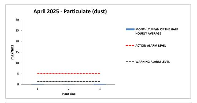
Following EA guidance and approval in July 2015, RRRL now monitor particulate emissions qualitatively as opposed to quantitatively. The Half Hourly and Daily ELVs no longer apply, the ELVs have been replaced by two alarm levels that prompt the operator to start an investigation or take further action these are set at: 1.5 mg/m3 – Warning Alarm and 5mg/m3 – Action Alarm.
